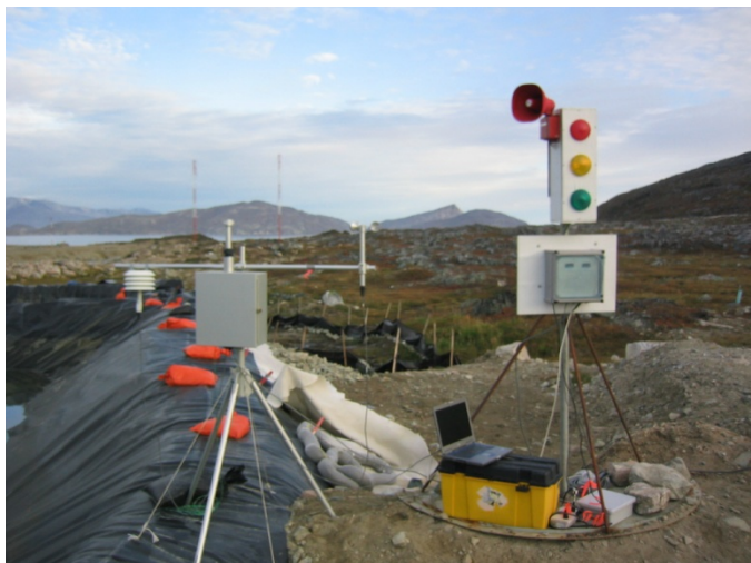
Figure 1. Continuous monitoring and alert system next to a soil remediation site. The warning system in the photograph had visual and audible alarms to alert the on-site manager to take mitigative action if airborne dust concentrations exceeded pre-established levels. We have implemented three such multi-site systems over the last 4 years.
